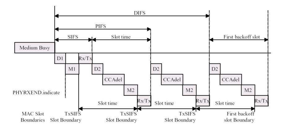
$\begin{array}{l} D1 = aRxRFDelay + aRxPLCPDelay (referenced from the end of the last symbol of a frame on the medium) \\ D2 = D1 + Air Propagation time \\ Rx/Tx = aRXTXTurnaroundTime (begins with a PHYTXSTART.request) \\ M1 = M2 = aMACPrcDelay \\ CCAdel = aCCATime - D1 \end{array}$
