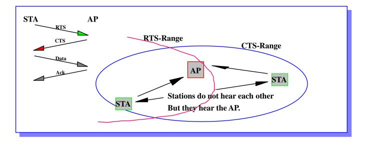
Separate Control frame exchange (RTS / CTS) between transmitter and receiver will *Reserve the Medium* for subsequent data access.
